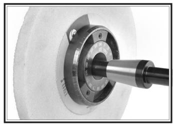
Figure 41. Installing the balancing arbor.
